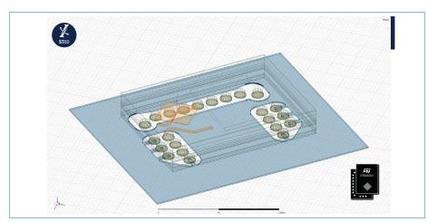
STMicroelectronics utilizes Ansys HFSS, a 3D electromagnetic (EM) simulation software for high-frequency electronics, to design and validate its 60GHz contactless communications products.
